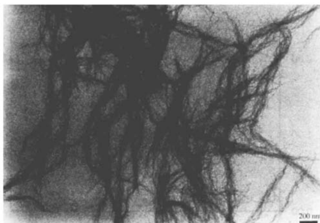
Fig. 3 Electron micrograph of micellar fibres made of 1c without staining
